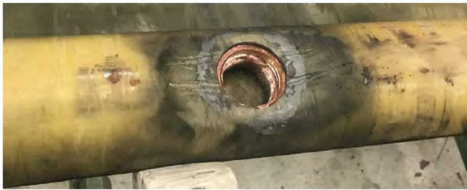
Damaged threads with raised metal
