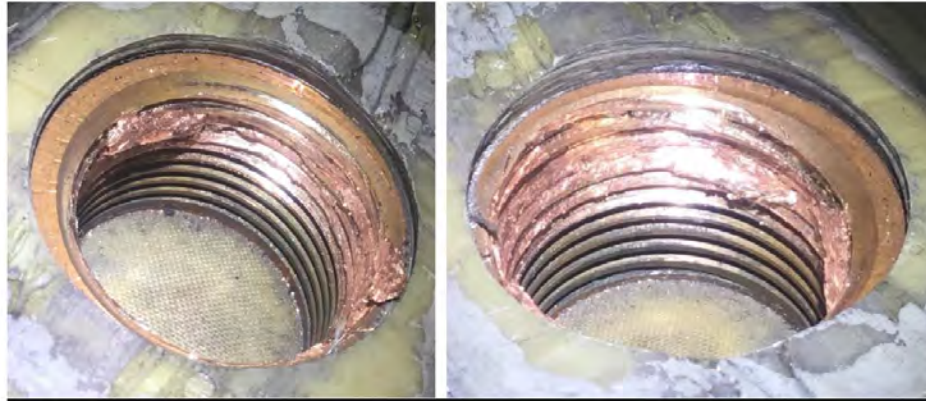
Damaged threads with raised metal
