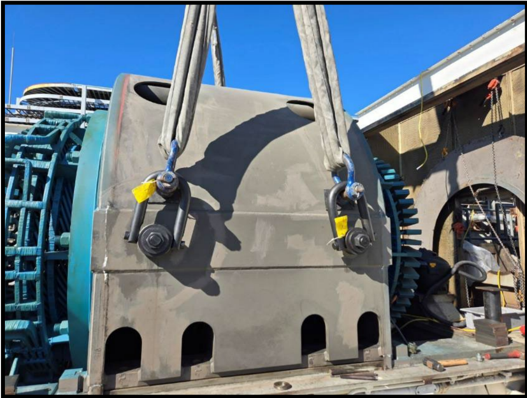
Stator to be rewound S/N 290T262 (Outer frame removed)
