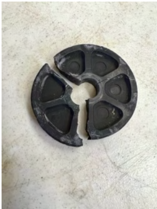
All 4 wheels broken on breaker
