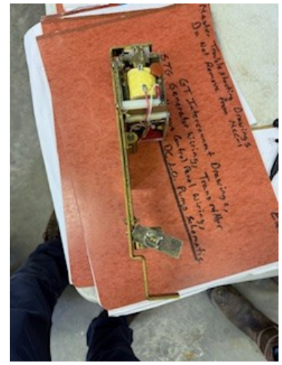
Bad under voltage relay
